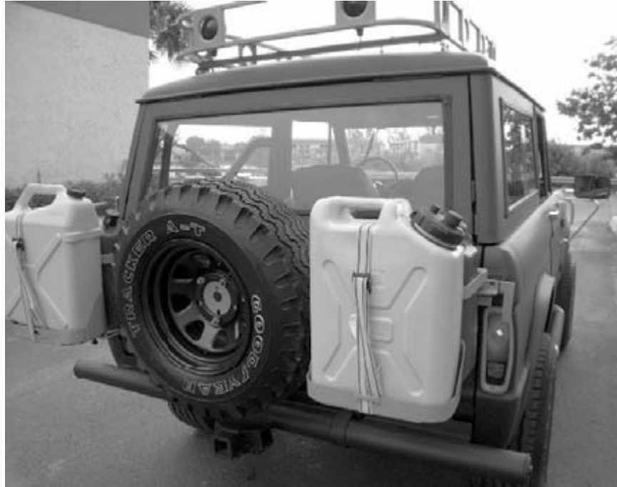
Fuel Storage Rack
