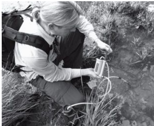
Pump Filter System
