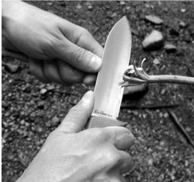
Stabilizing Knife With Thumb While Carving
