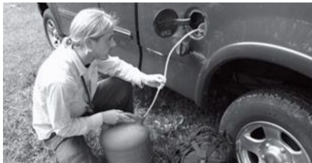
Tubing as Fuel Siphon
