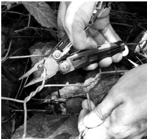
Cutting Fence With Multi-Tool Wire Cutters
